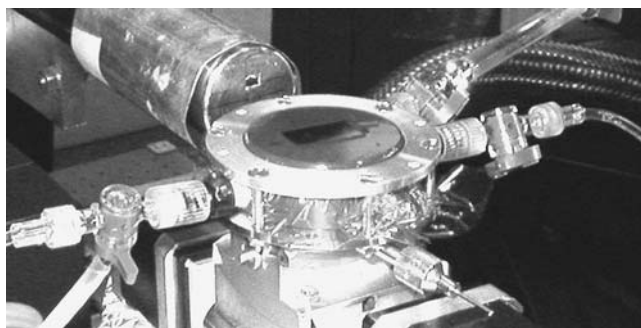
FIGURE 2 Photograph of liquid-solid interface cell. The Kapton film is sealed against the substrate holder by an annular aluminum ring with the Si/Mo x-ray mirror substrate in the center. The grazing angle incident beam direction is along the length of the sample. The three valves are used for injecting and withdrawing aqueous solutions. The solid-state x-ray fluorescence detector collects x-rays that are emitted from the sample surface through a small window aperture in a Pb cap that covers the detector.
